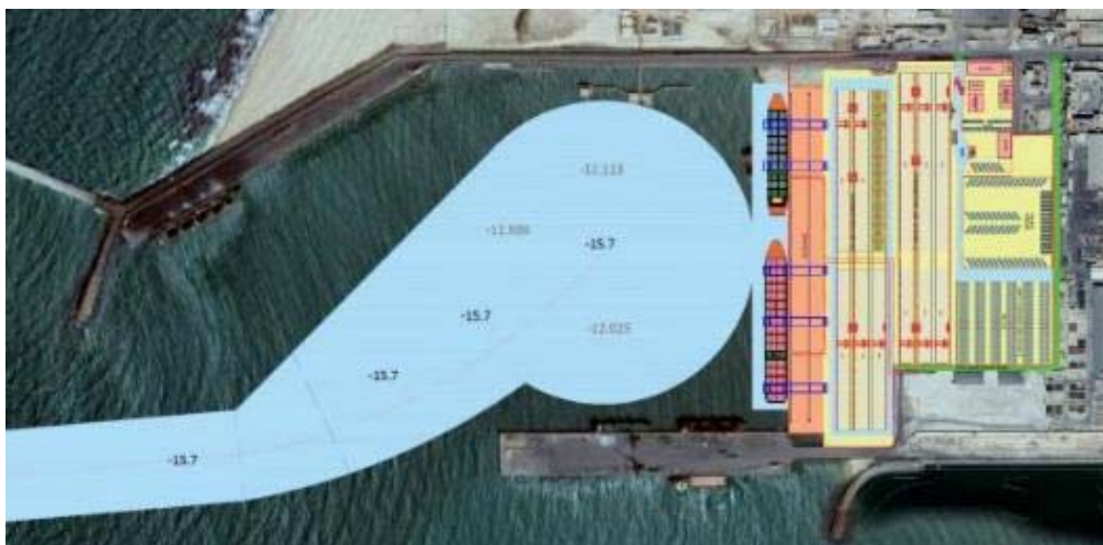
Figure 3-7: Conception préliminaire des composantes de la phase 2 (Plan No. NCT-EPC-1001-SHEET-1, November 2018, Afcons)
